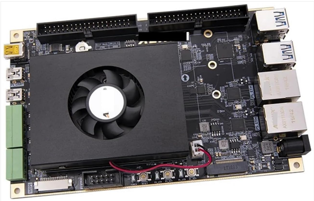
A top-down view of the AXU3EGB board, highlighting the integrated cooling solution for the main processing unit.
