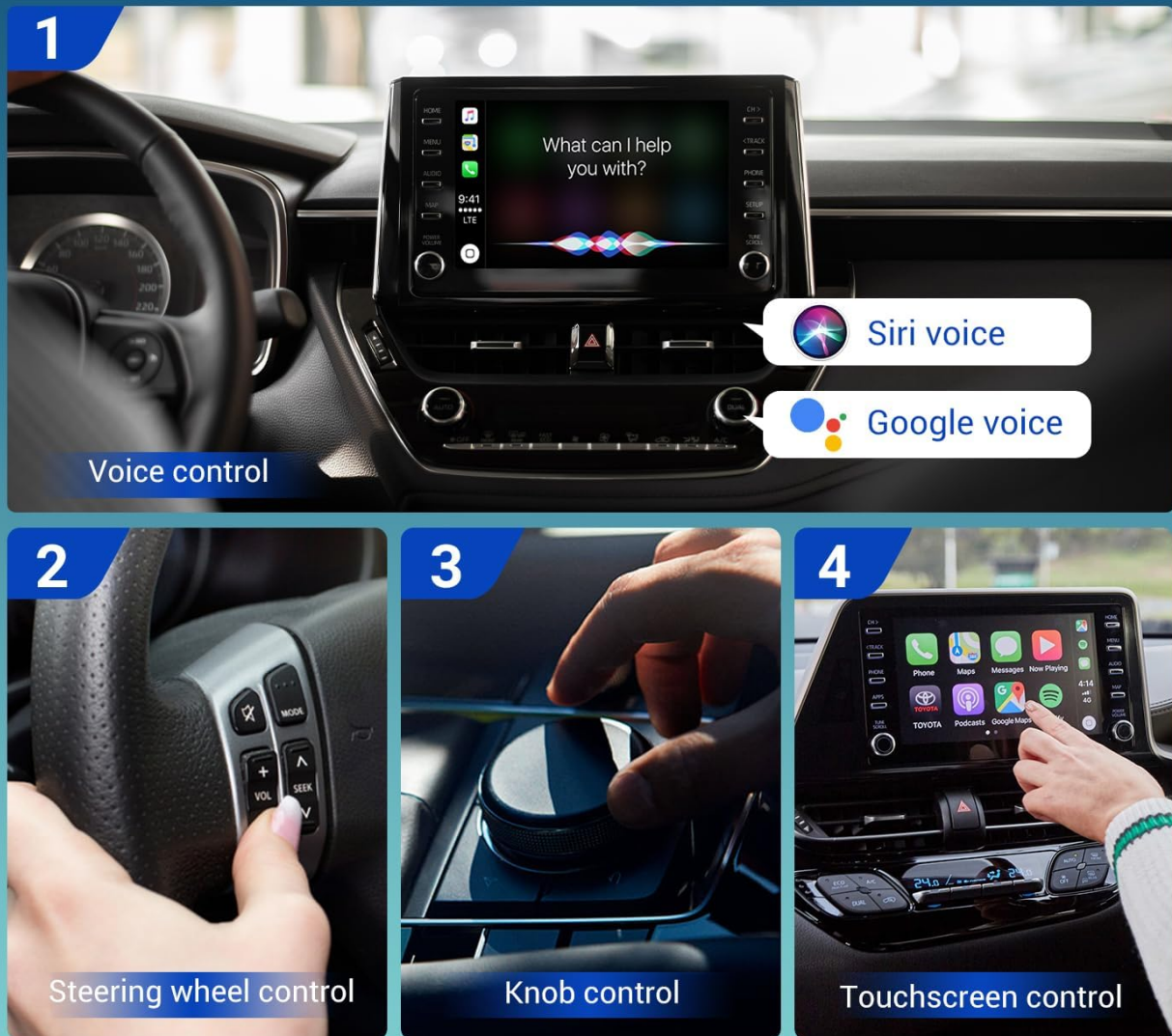
Figure 4: The adapter maintains compatibility with your vehicle's original control systems for a familiar user experience.
