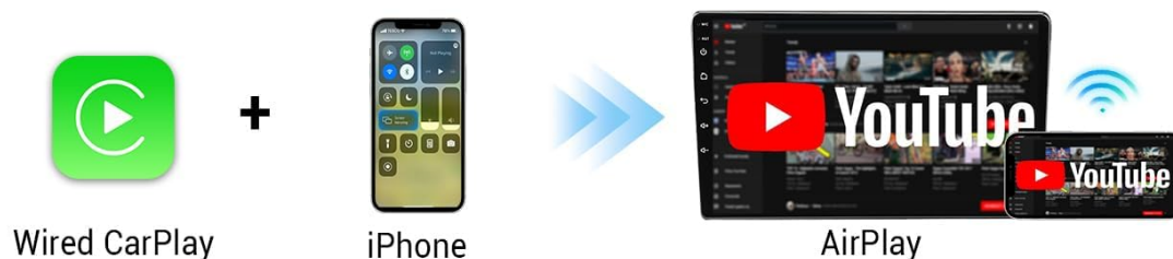
Figure 1: The OTTOCAST MX adapter offers 3-in-1 functionality, converting wired CarPlay to wireless CarPlay, wired Android Auto to wireless Android Auto, and wired CarPlay to AirPlay.
