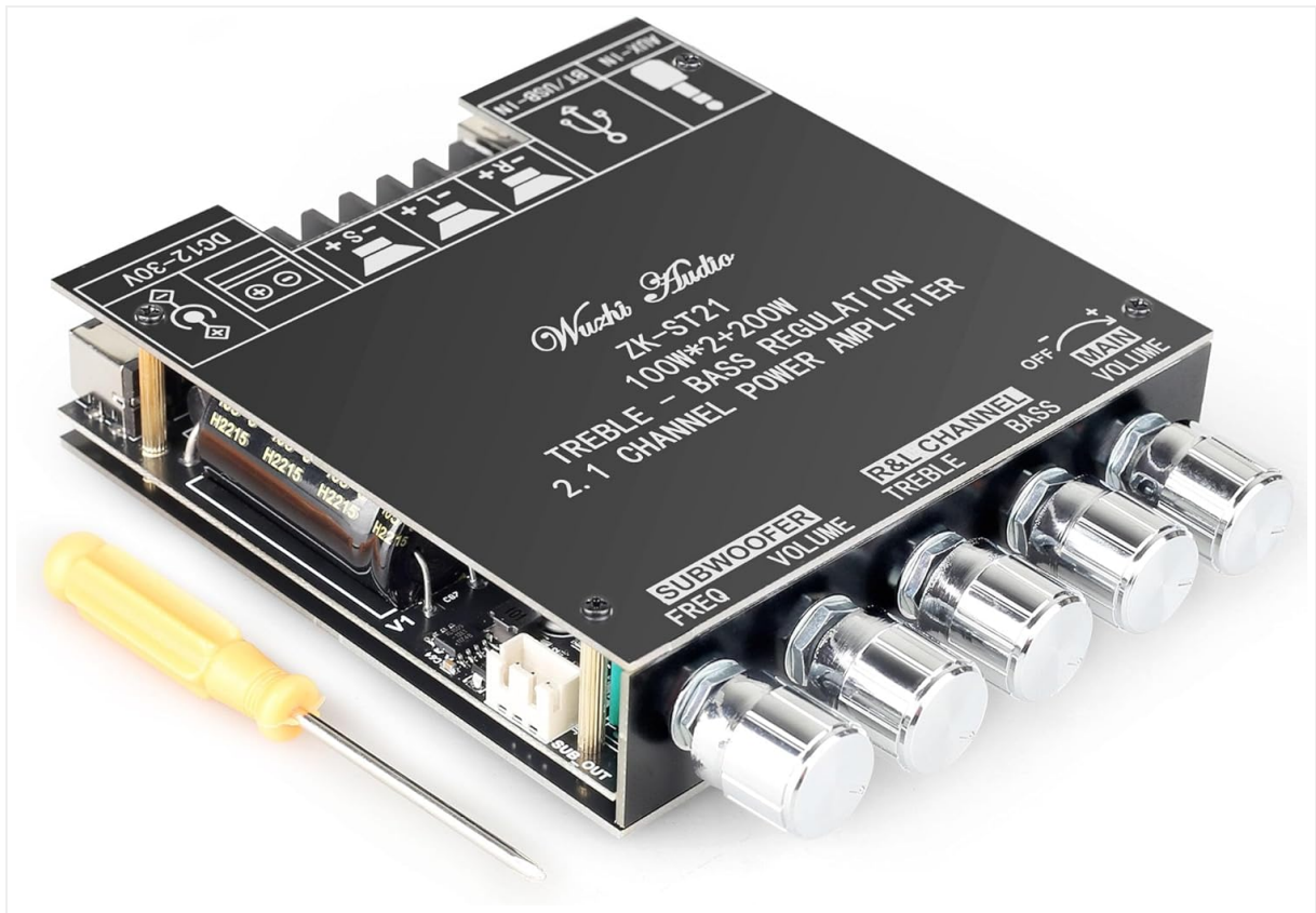
Figure 1: DAJUNGUO ZK-ST21 TPA3221 Bluetooth Power Amplifier Board with screwdriver for assembly.
