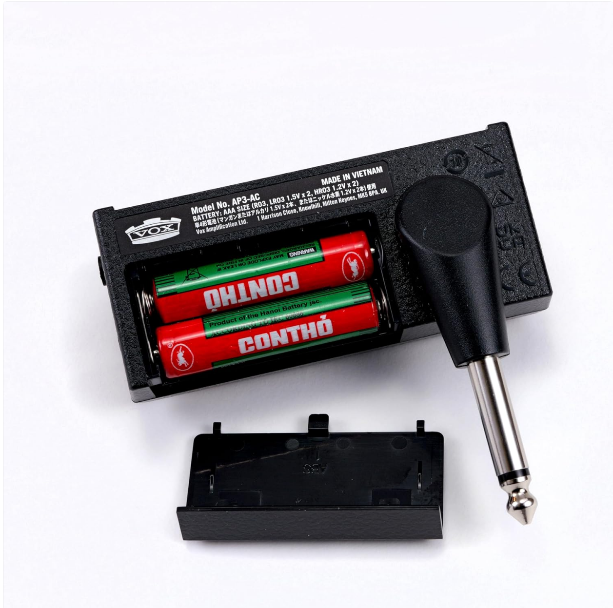
Image 3.1: The battery compartment of the amPlug 3, showing the placement of two AAA batteries.
