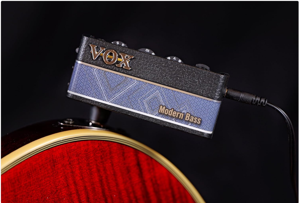
Image 3.2: The amPlug 3 Modern Bass connected to the output jack of a bass guitar.
