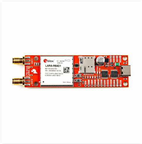
Angled view of the SparkFun LTE Stick, highlighting the two SMA antenna connectors and the USB-C port.
