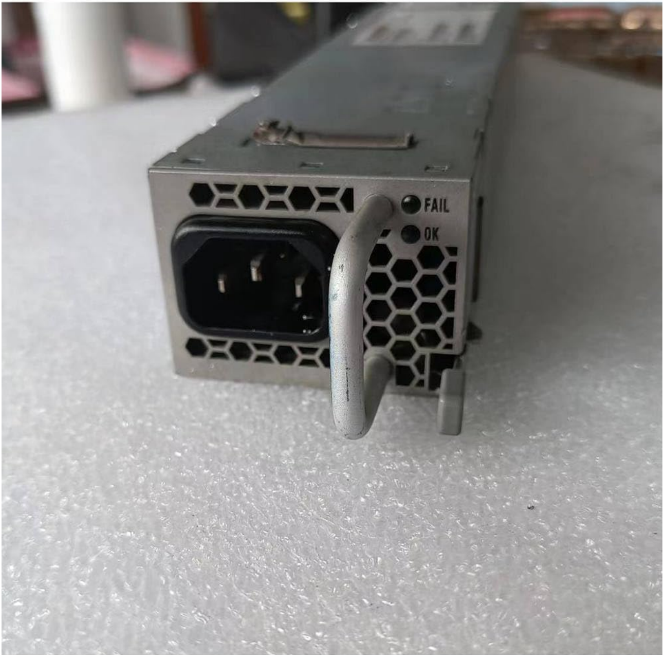
Figure 3.4: Front panel of the power supply, featuring the standard IEC C14 AC power inlet and two LED indicators: 'FAIL' (red) and 'OK' (green), which indicate the operational status of the unit.
