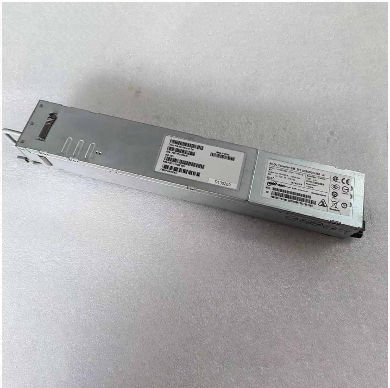
Figure 4.1: Side view of the power supply, demonstrating its compact form factor suitable for hot-swappable installation in compatible network switches or servers.
