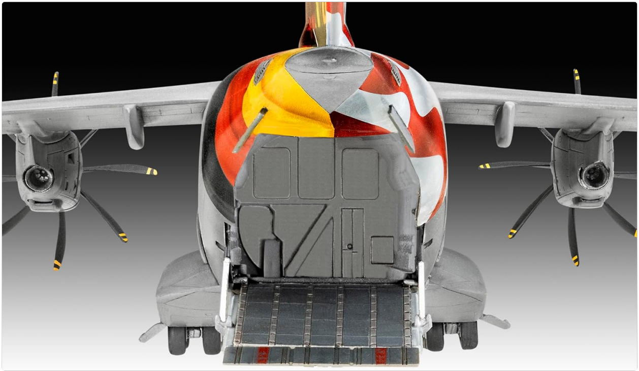
Figure 3.3: The Airbus A400M model's rear cargo bay, depicted in an open position with ramp details.
