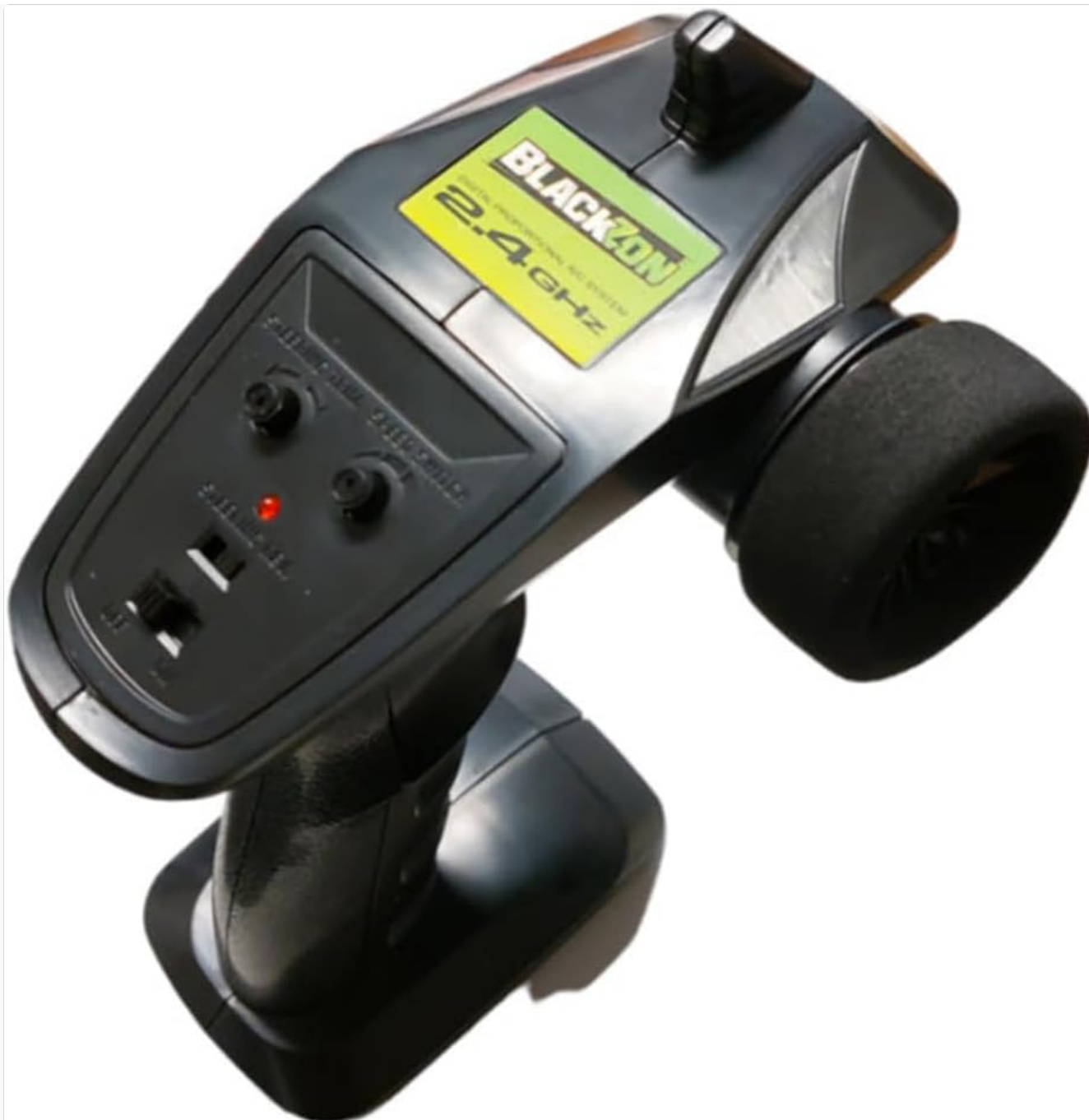
Figure 4.4: Top view of the 2.4GHz radio transmitter, showing the various adjustment dials and power switch.
