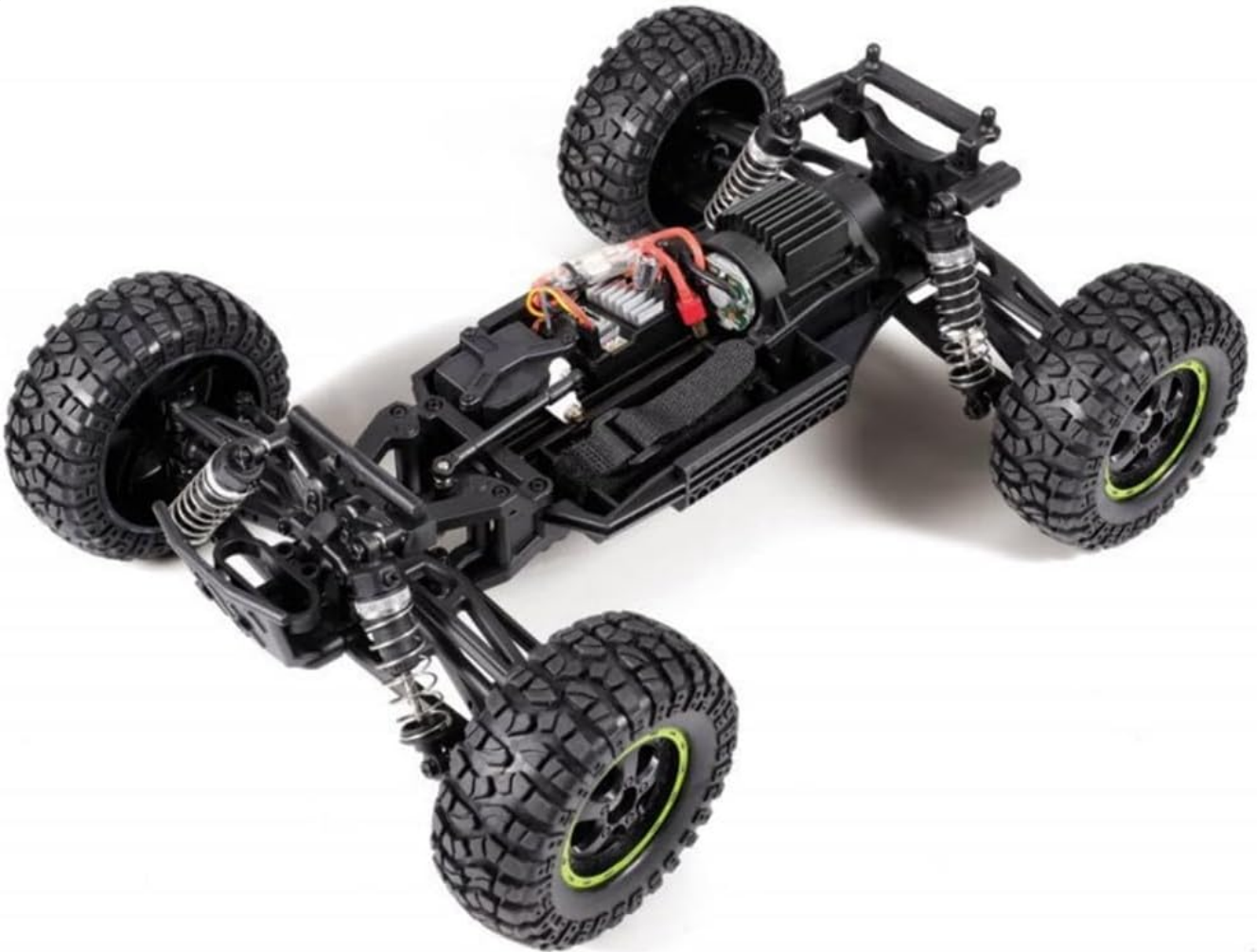
Figure 4.2: Top-down view of the BlackZon Smyter MT Turbo chassis with the body removed, showing the internal electronics, motor, and drivetrain components.
