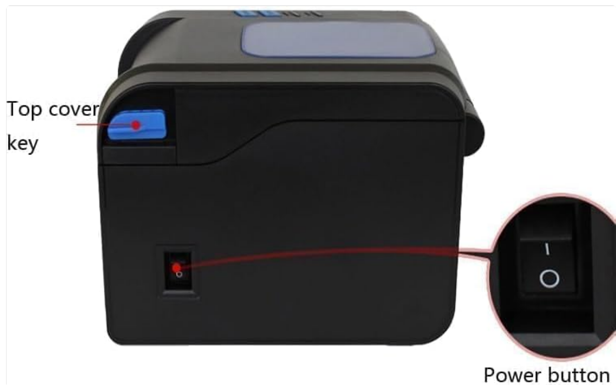
Figure 4.2: Side view illustrating the power button and top cover key for accessing the media compartment.
