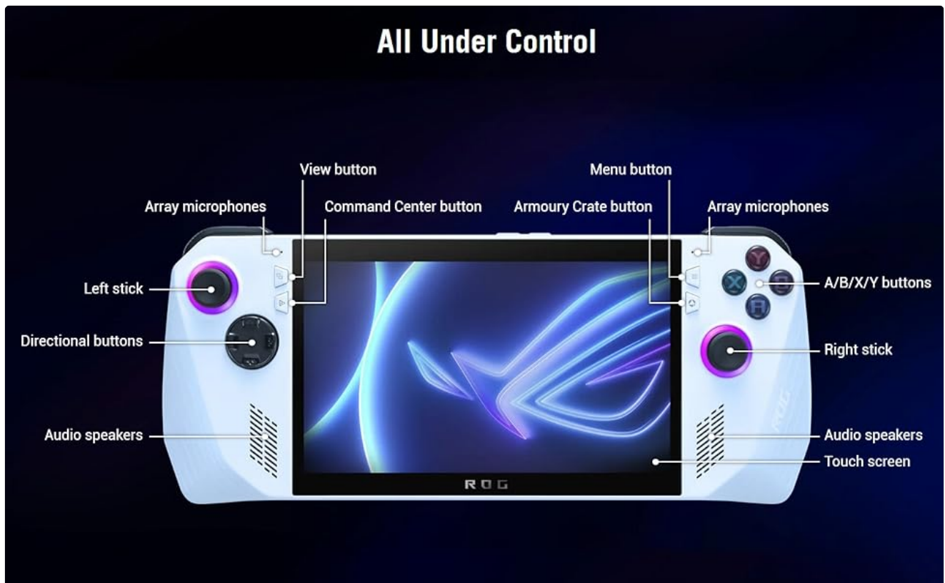
Figure 2.2: Front view of the ROG Ally with key controls labeled, including the 7-inch touchscreen, left and right sticks, directional buttons, A/B/X/Y buttons, View button, Menu button, Command Center button, Armoury Crate button, and array microphones.
