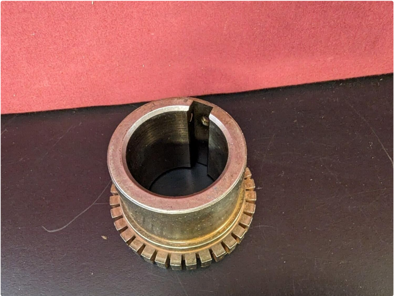
Image 4: Top-down view of the Falk 1040T Hub, showing the central bore and the external gear teeth designed to engage with the flexible element of a Steelflex coupling. Markings on the hub indicate "FALK 1040T" and a part number.
