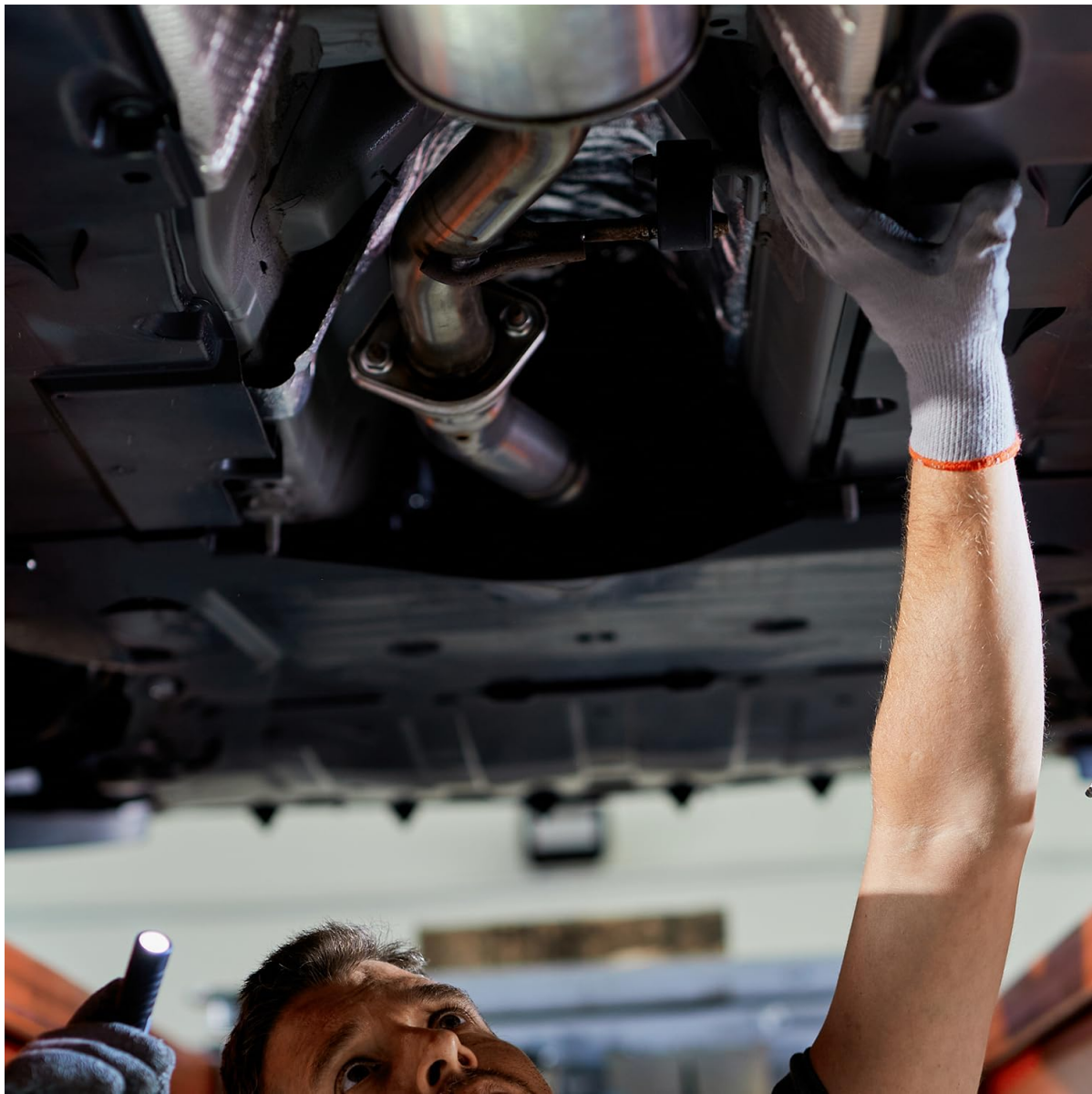
Image 3.2: A mechanic inspecting the DPF and catalytic converter area under a vehicle.
