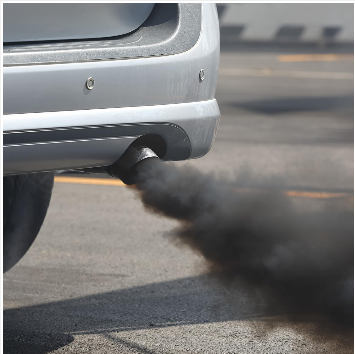
Image 4.2: Initial dark smoke from the exhaust, indicating soot and carbon being expelled during the cleaning process.
