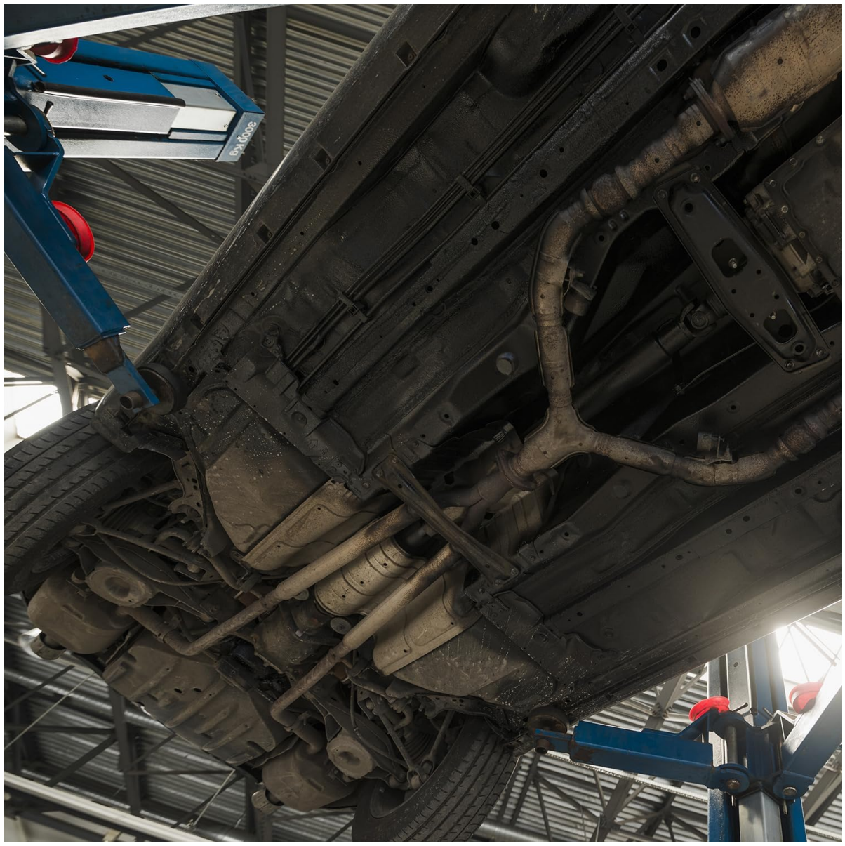
Image 3.1: Vehicle raised on a lift, providing access to the exhaust system for DPF cleaning.
