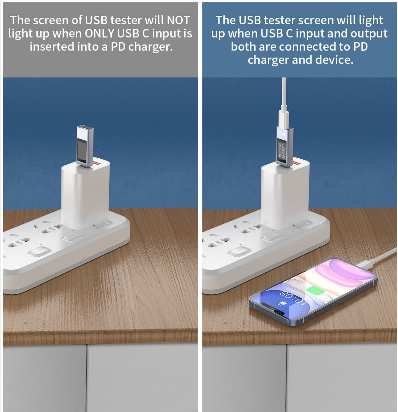
Figure 3.1: Correct connection method for PD chargers.
