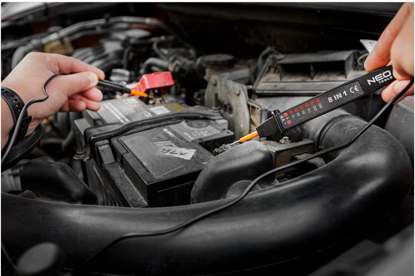
Figure 6: Using the tester to check voltage on a car battery.
