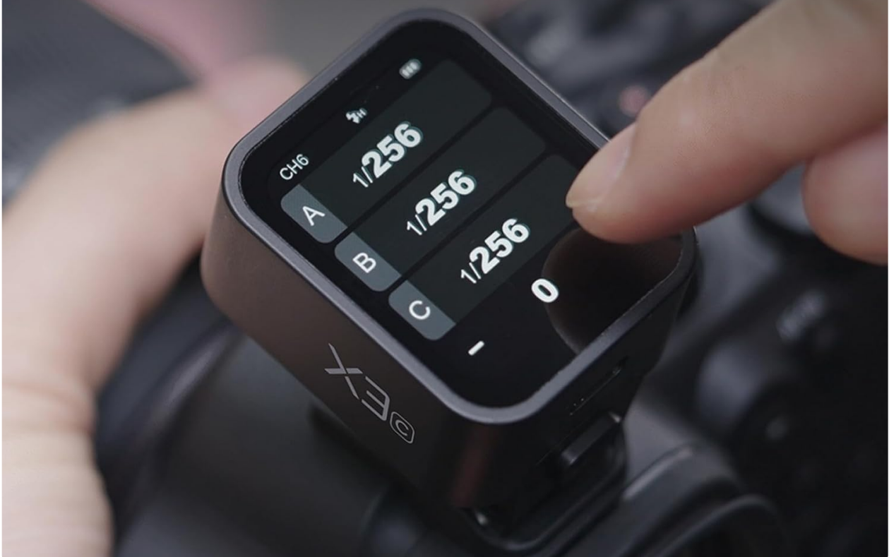
Image: A finger interacting with the X3C's touchscreen to change flash power settings.
