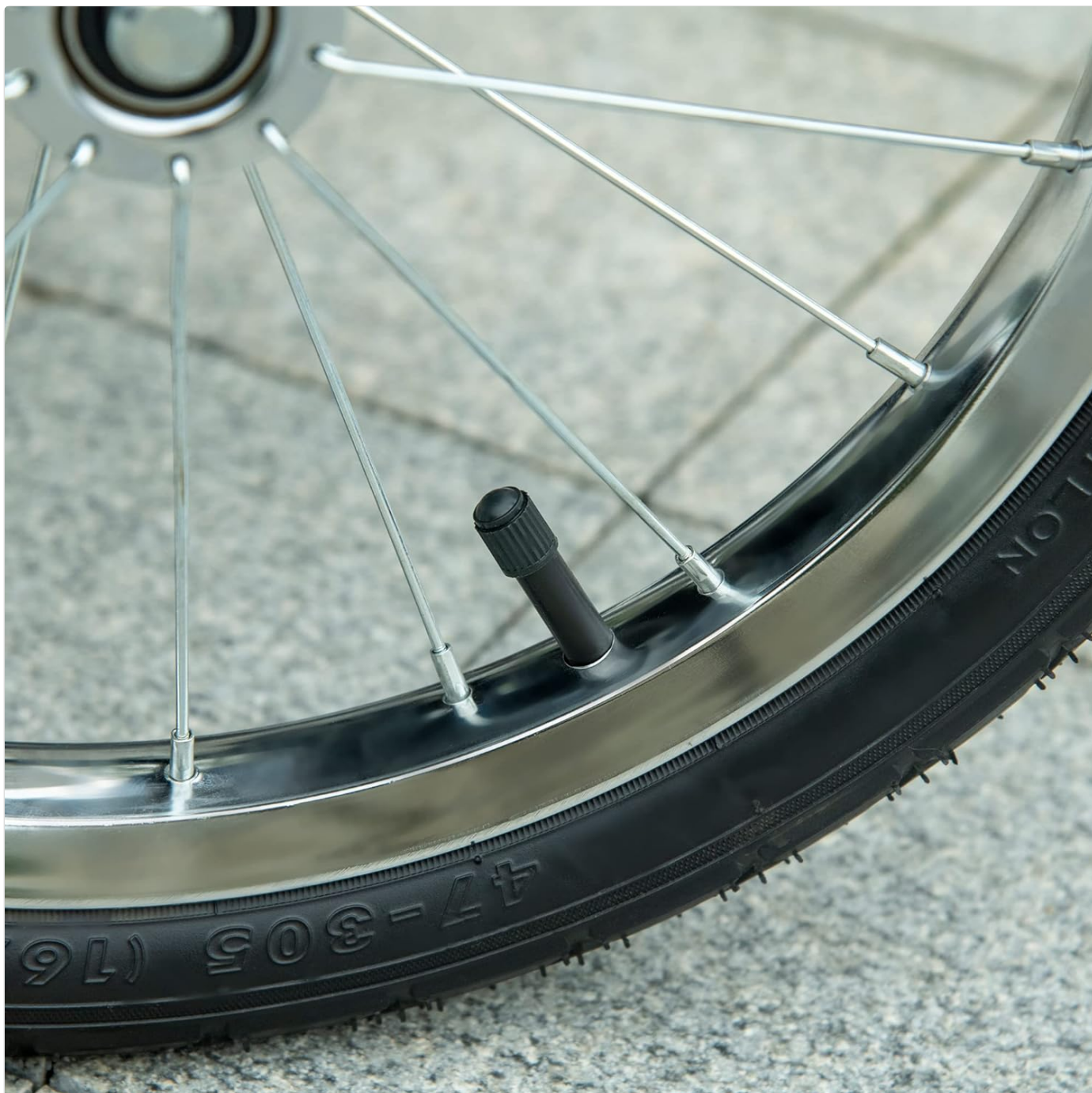
Image: Close-up of the tire valve, indicating the point for inflation.
