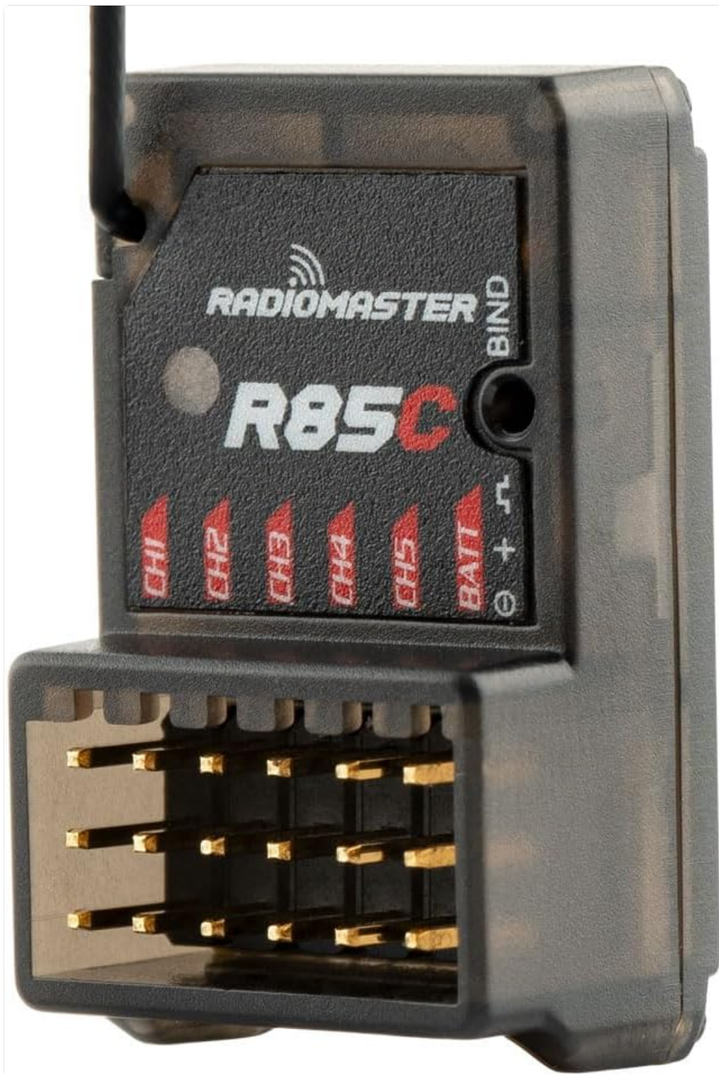
Figure 4.2: A detailed close-up of the Radiomaster R85C receiver's top surface, clearly showing the labels for channels CH1 through CH5, the BATT port, and the 'BIND' button.
