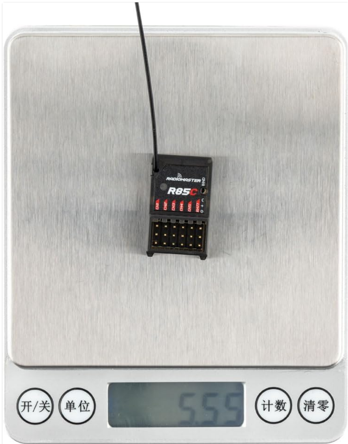
Figure 3.2: The Radiomaster R85C receiver placed on a digital scale, displaying a weight of 5.55 grams, confirming its lightweight design.
