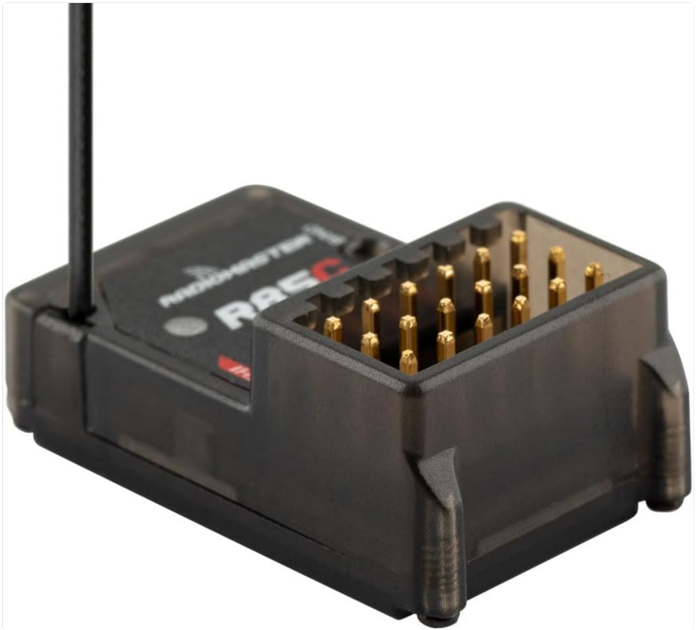
Figure 4.3: An angled view of the Radiomaster R85C receiver, showcasing the gold-plated pin headers for connecting servos and power, along with the integrated antenna.
