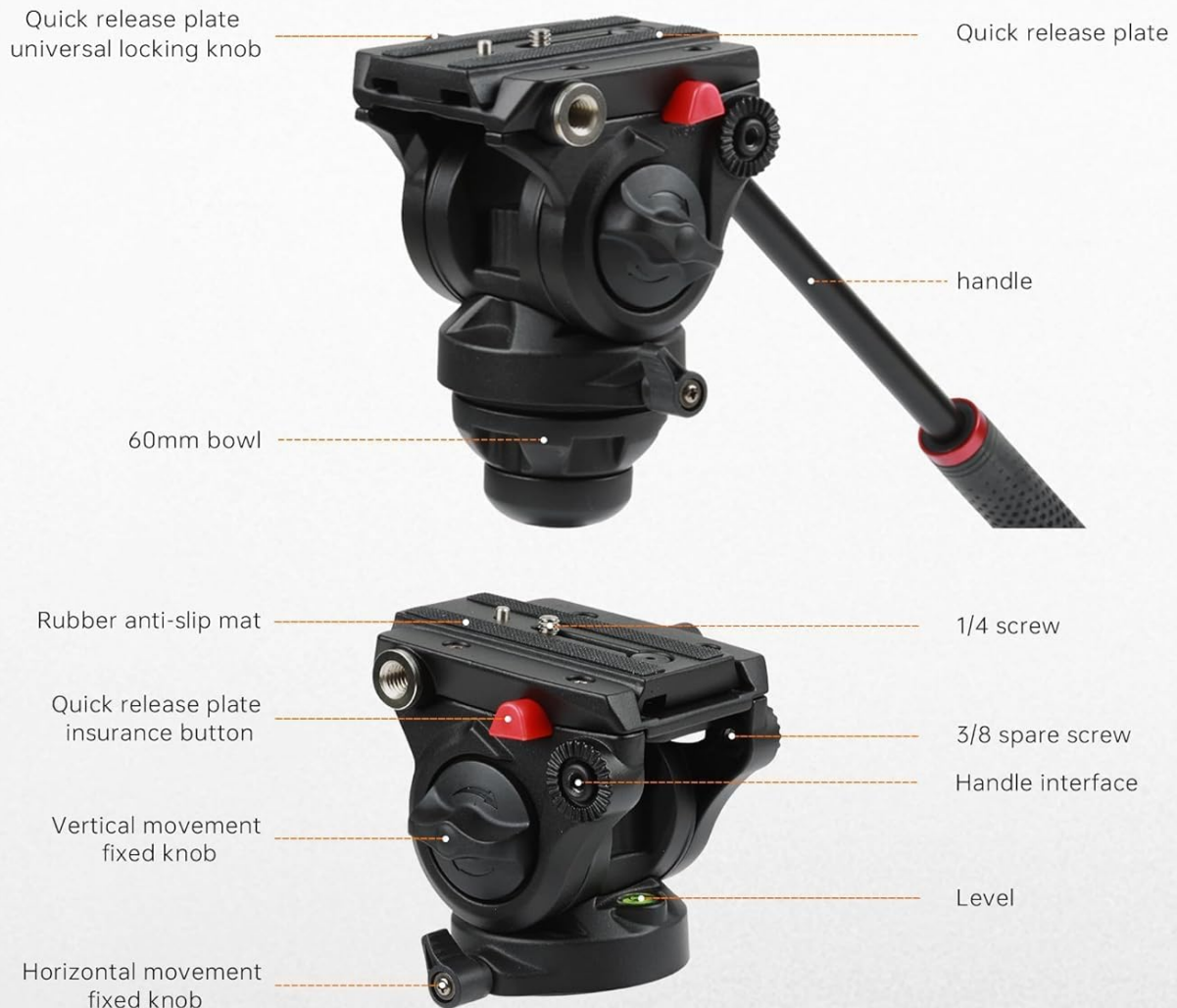
Image 3.1: Detailed view of the VT-01 Fluid Head, showing the quick release plate, handle, 60mm bowl, 1/4" and 3/8" screws, and various adjustment knobs.
