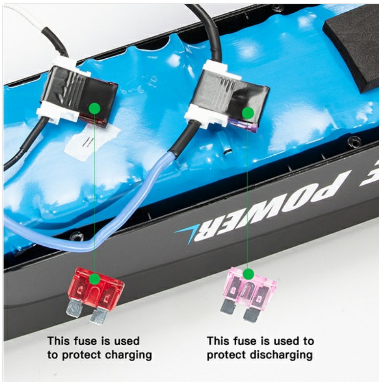
Image: Fuse locations for charge and discharge protection.
