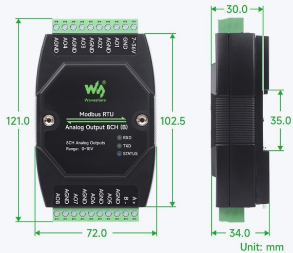
Image 12.1: Front, side, and top views with dimensions (e.g., 121.0mm length, 72.0mm width, 34.0mm depth).
