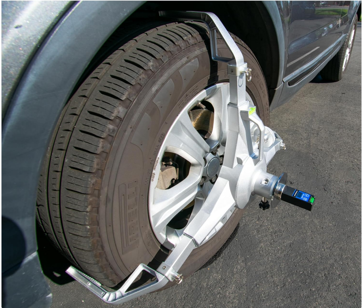
Figure 5: The tire clamp properly installed on a vehicle's tire.
