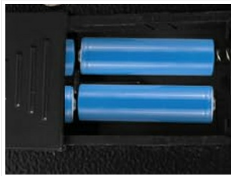
Figure 3: External battery box, which can be used for temporary power if internal batteries are depleted.
