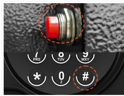
Figure 5: Location of the red reset button for passcode programming.
