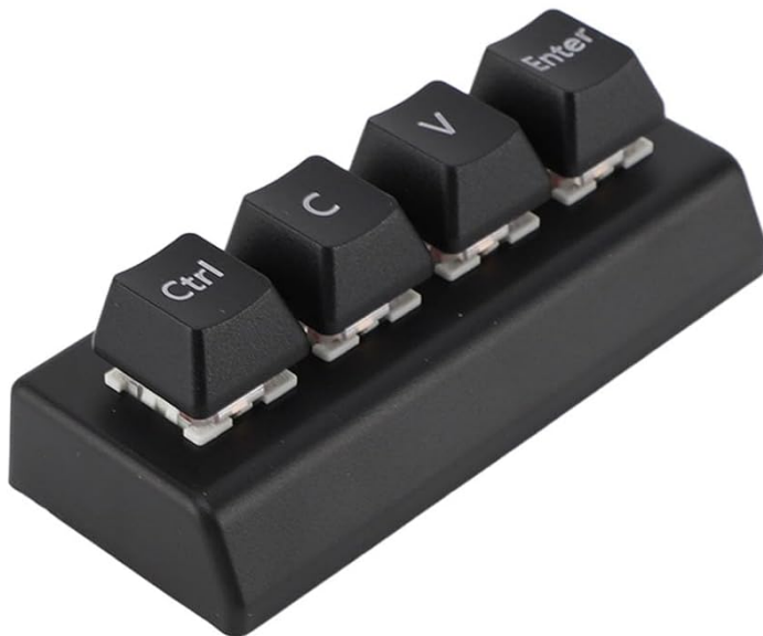
Image 5.1: The keypad illustrating its programmable design. Repetitive settings are allowed, and configurations are saved on the device, eliminating the need for re-setting when changing devices.
