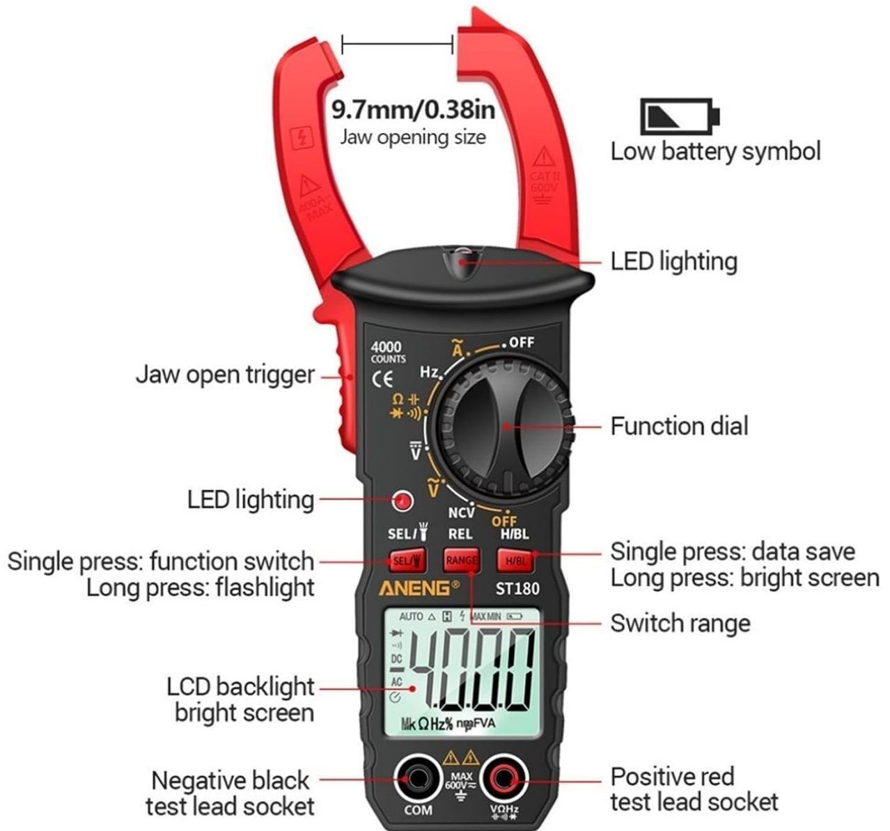
Figure 2: Labeled components of the ST180 Clamp Meter.
