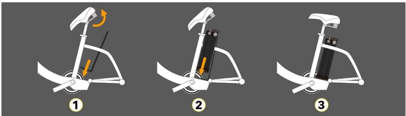
Image 4.2: Visual guide for installing the battery onto the bicycle seat tube.
