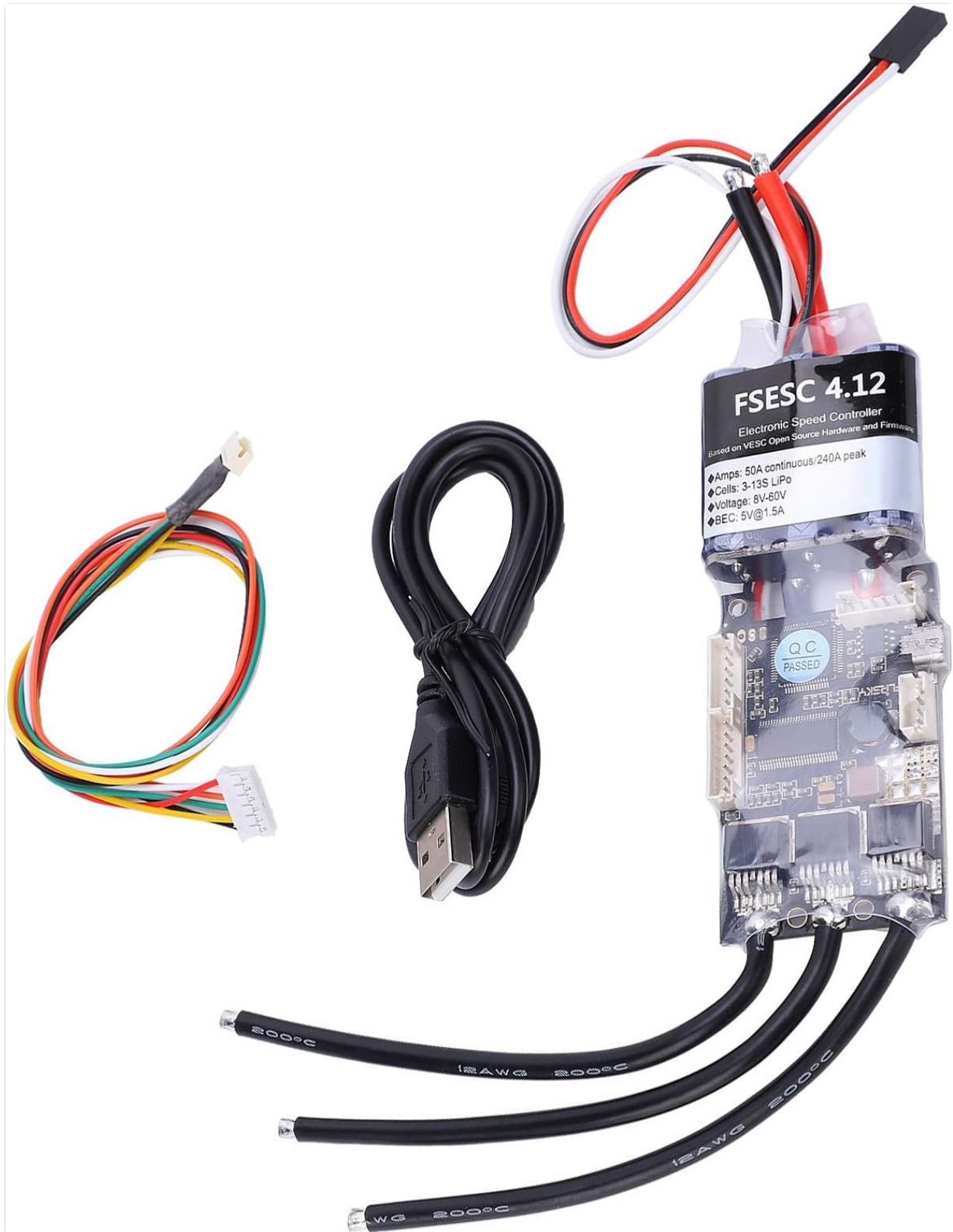
Image 2.1: The Fafeicy Flipsky ESC V4.12 Electronic Speed Control, shown with its accompanying USB cable and VESC sensor line.
