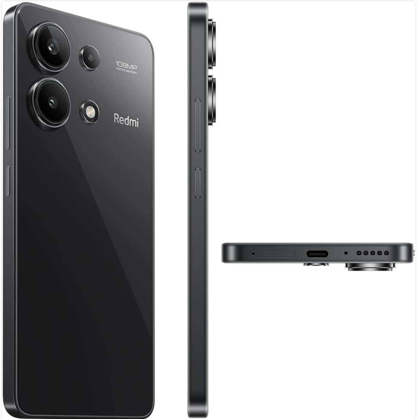
Image: Side and top/bottom views of the Redmi Note 13 4G LTE, illustrating the location of the SIM tray and USB-C port.
