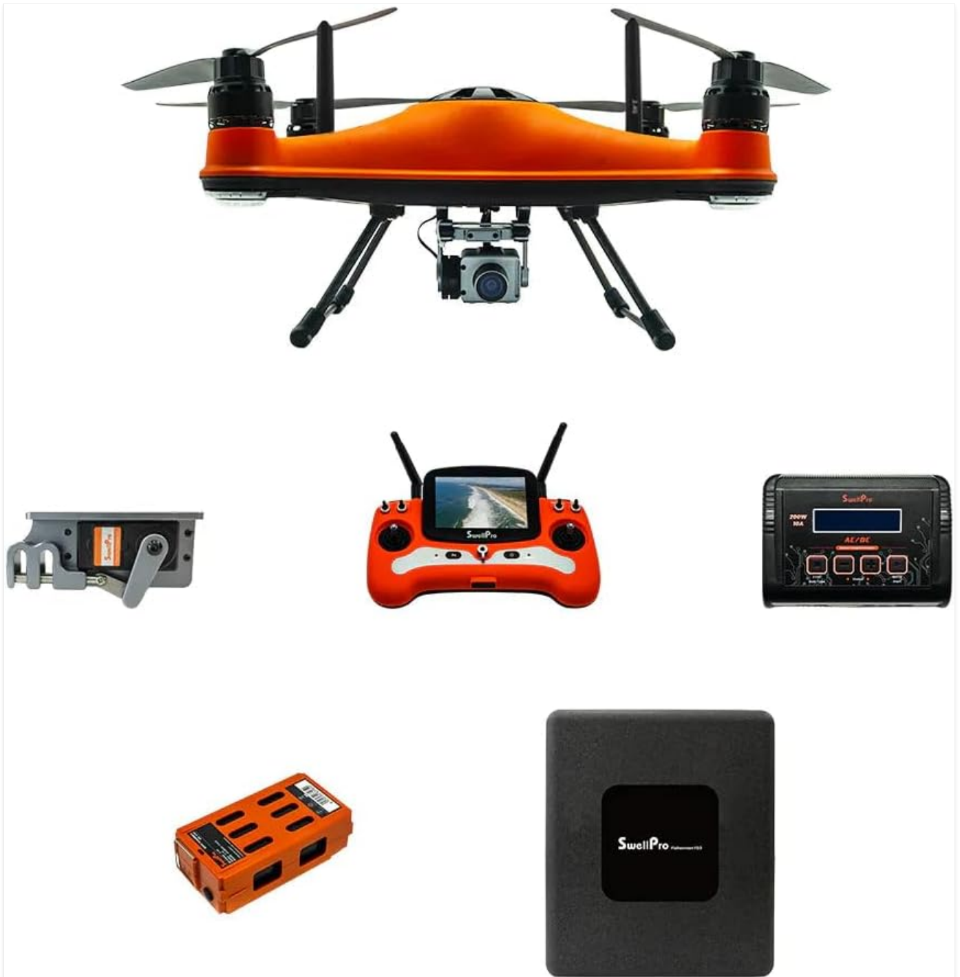
Figure 2.1: The SwellPro FD3 Fisherman drone shown with its primary accessories, including the remote control, flight battery, charger, and bait release mechanism.
