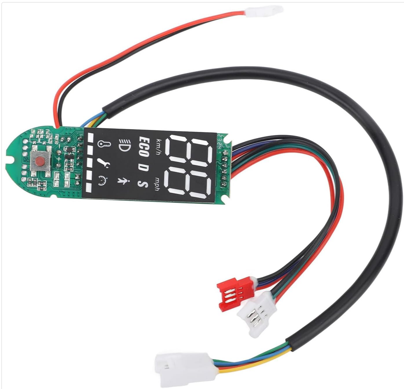
Figure 4: A close-up view of the dashboard's digital display, showing speed (88), unit (km/h or mph), and various status icons like ECO, D, S, and a light indicator.
