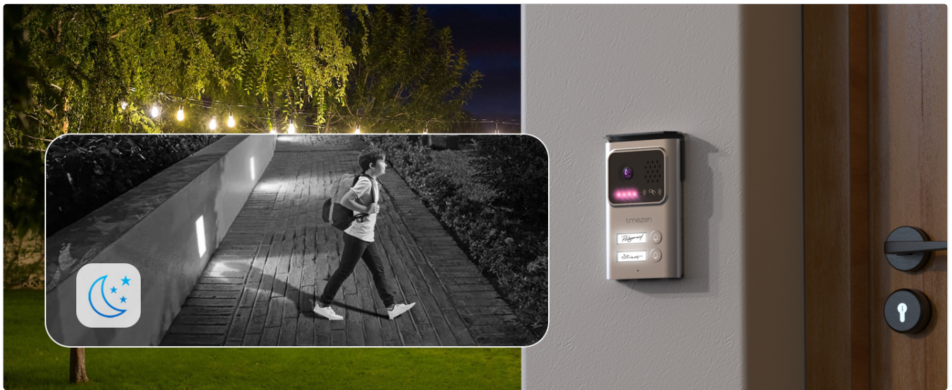
Figure 5.14: The outdoor doorbell unit's night vision capability, showing a clear image in a dark outdoor setting.
