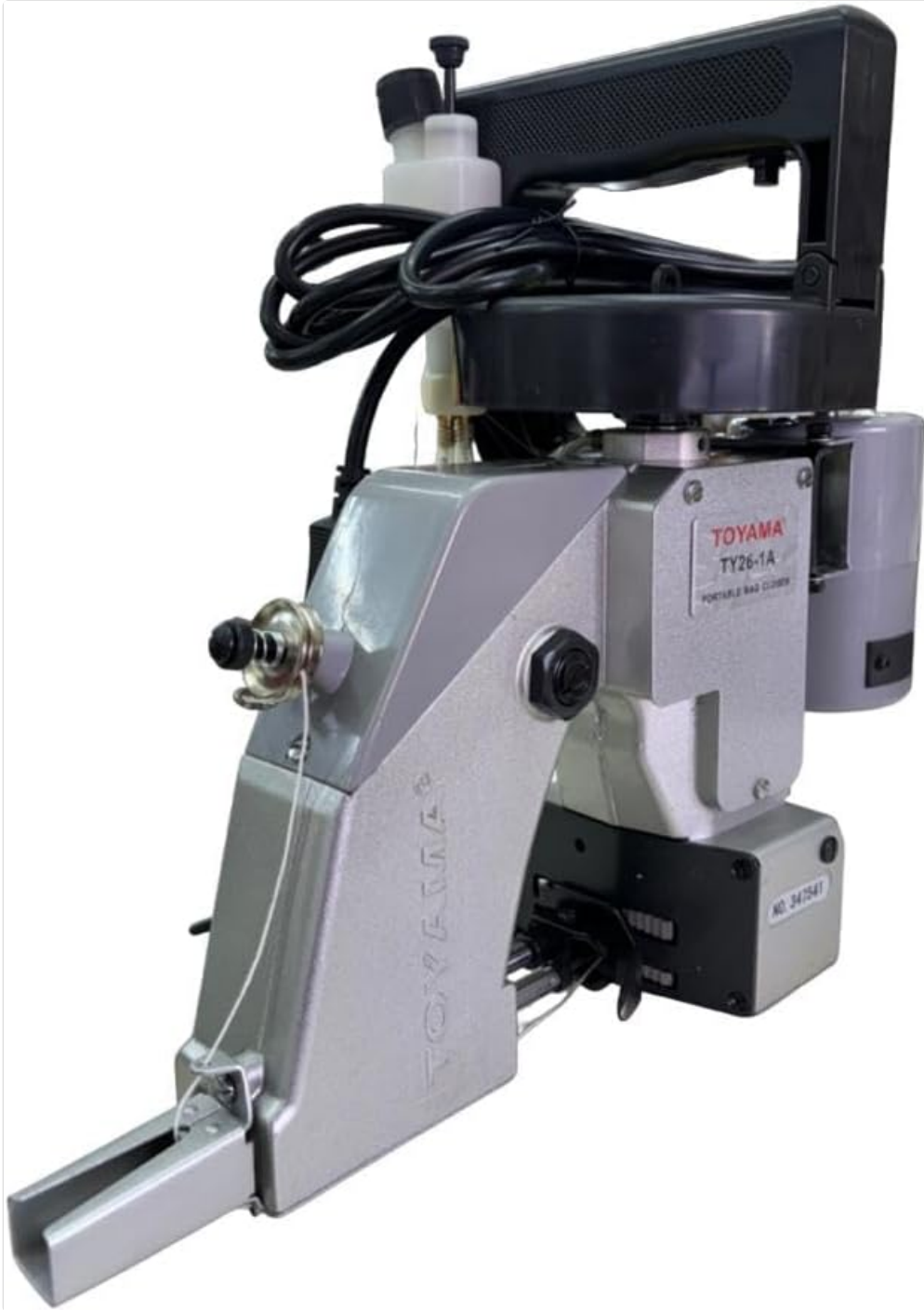
Figure 4.1: Front-side view of the Toyama Portable Bag Closer Sewing Machine, highlighting the handle and model number TY26-1A.
