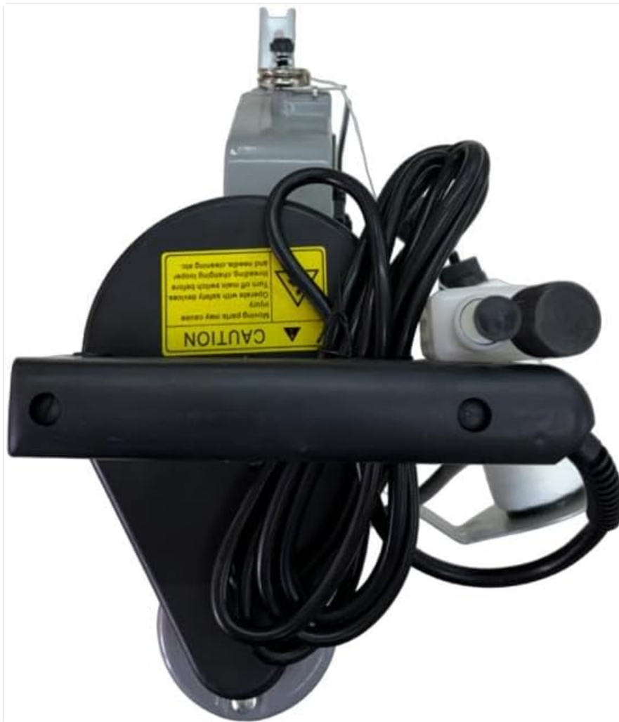
Figure 4.3: Side view of the Toyama Portable Bag Closer Sewing Machine, showing the power cord and oil reservoir.
