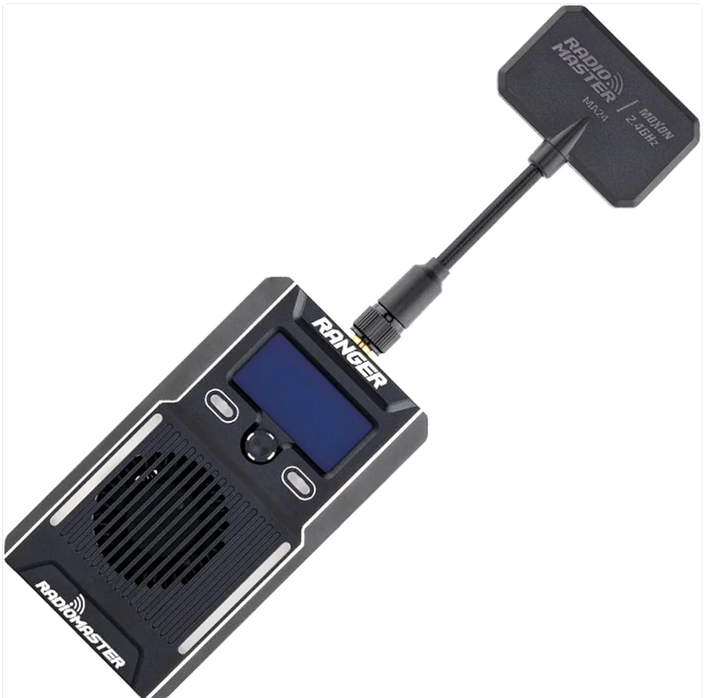
Figure 4.1: Front view of the Ranger module with the Moxon antenna attached, showing the OLED display and control buttons.
