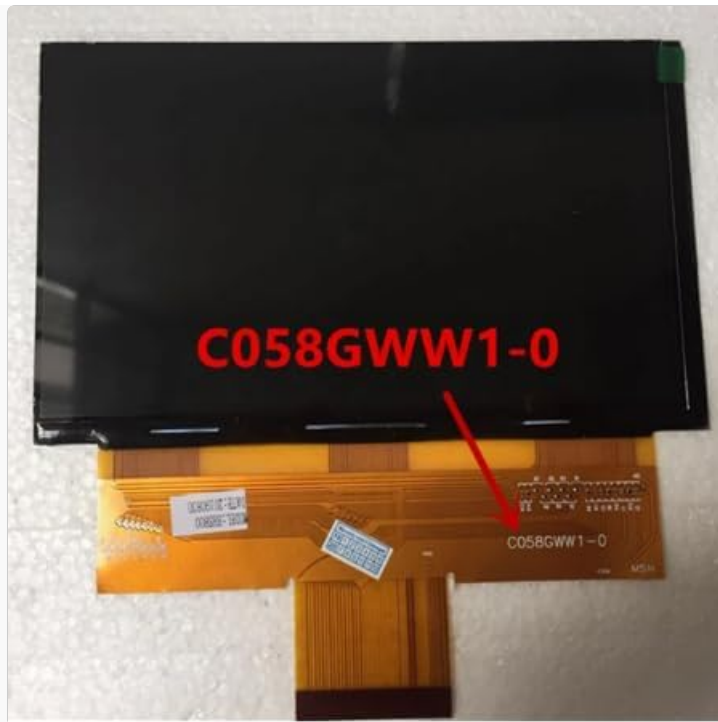
Figure 3: C058GWW1-0 LCD Display Module, illustrating its compact design and connector.
