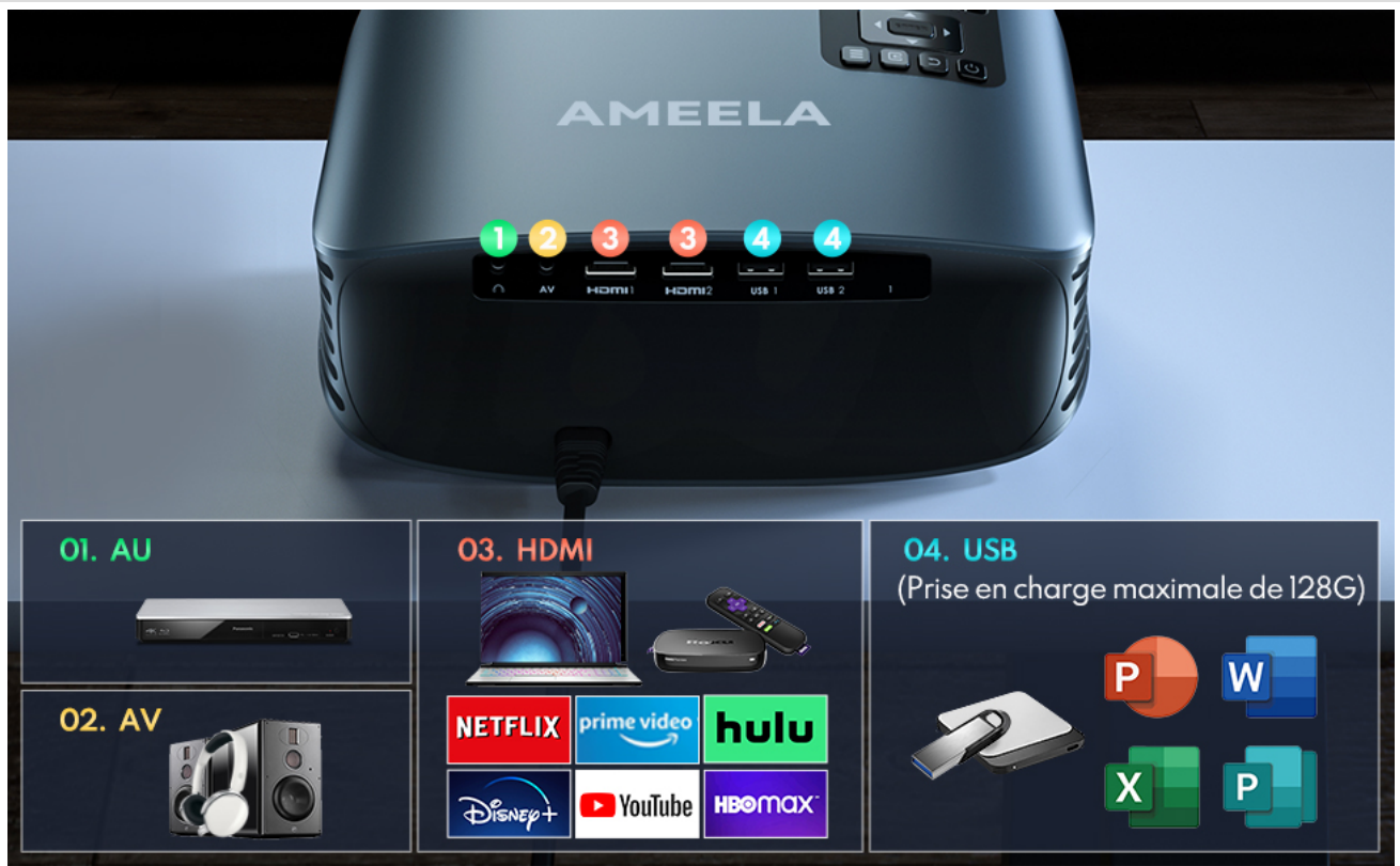
Image: Close-up view of the projector's input panel, showing ports for Audio Out (AU), AV, HDMI (HDMI1, HDMI2), and USB (USB1, USB2) with examples of compatible devices.
