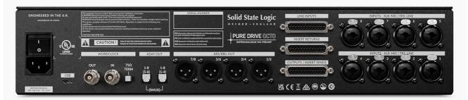
The rear panel provides all input and output connections. This includes XLR/TRS combo jacks for microphone/line inputs, D-Sub connectors for line inputs and outputs/sends, ADAT and AES/EBU digital outputs, Wordclock I/O, and a USB port for computer connectivity. The power inlet is located on the far left.
