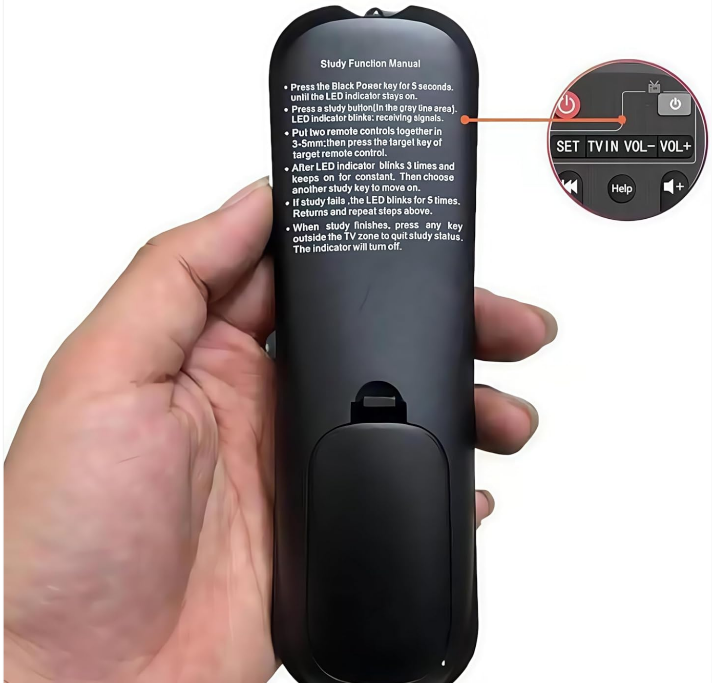
Image: Back view of the BIFANS remote control, highlighting the battery compartment and providing a visual guide to the learning function steps.
