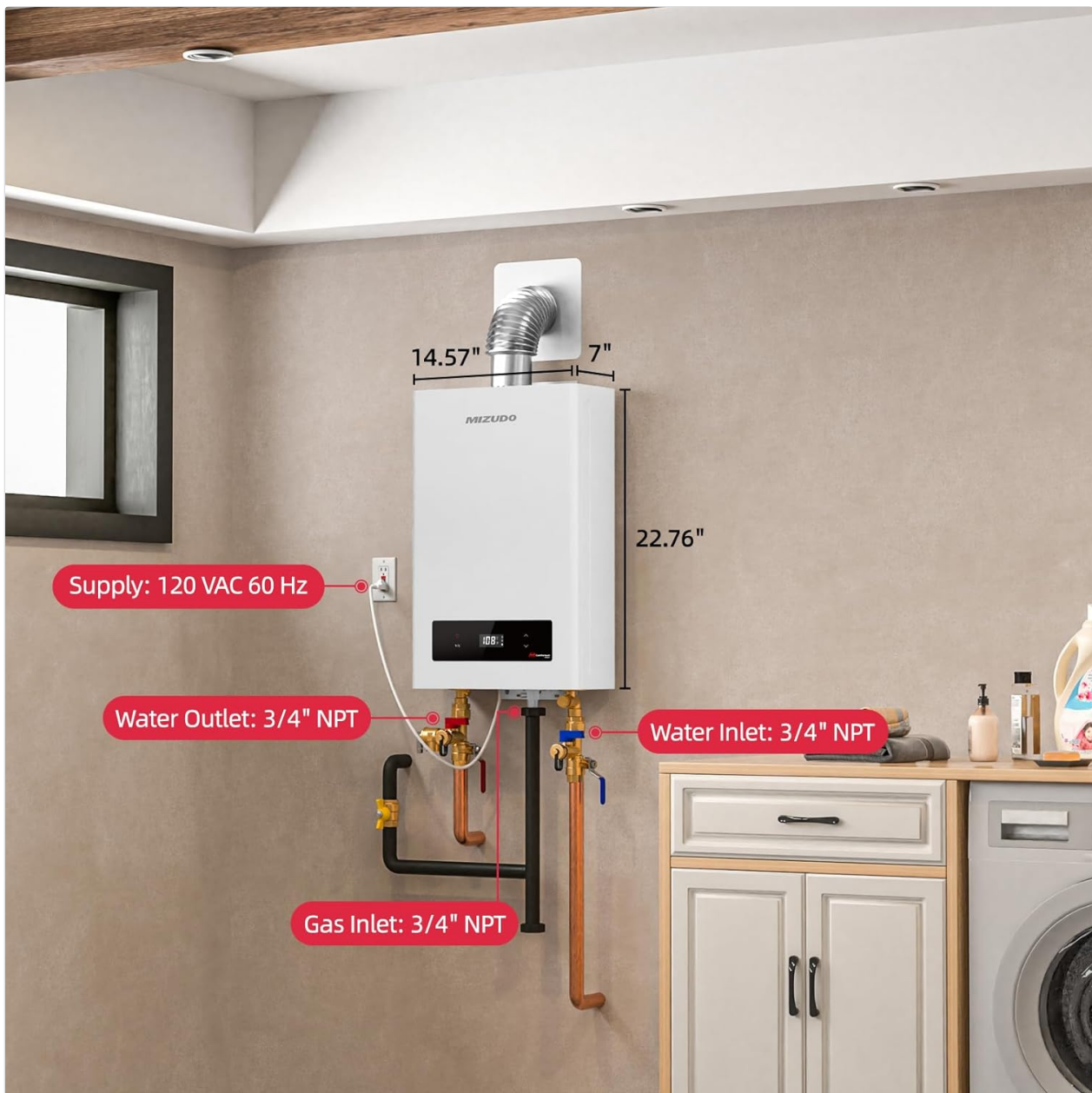
Figure 6: Installation Diagram. This diagram illustrates the physical dimensions of the unit (22.76"H x 14.57"W x 7.0"D) and the required connection points for 120V AC power, 3/4" NPT water inlet, water outlet, and gas inlet.
