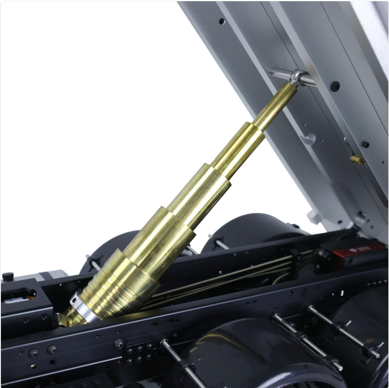
Image: A detailed view of the hydraulic cylinder responsible for lifting and lowering the dump bed.
