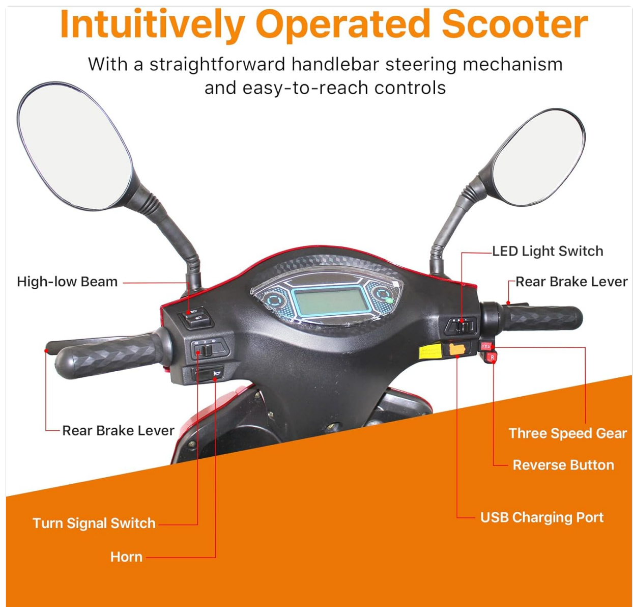
Figure 2: Detailed view of the scooter's control panel, highlighting various switches and indicators.
