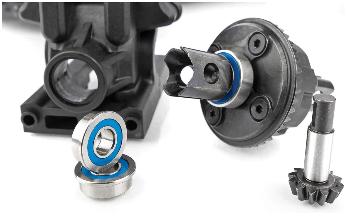
Figure 2.4: Components of the drivetrain, including the differential, bearings, and various gears.
