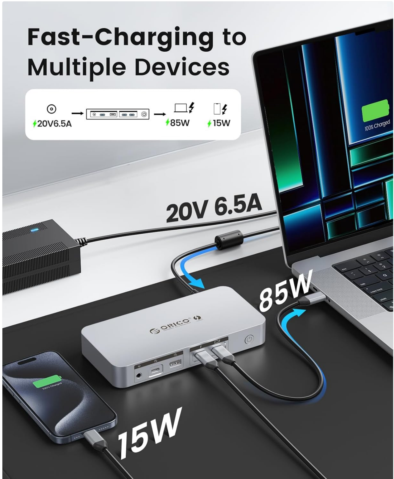
Figure 3: Connecting the docking station for power and host device charging.
