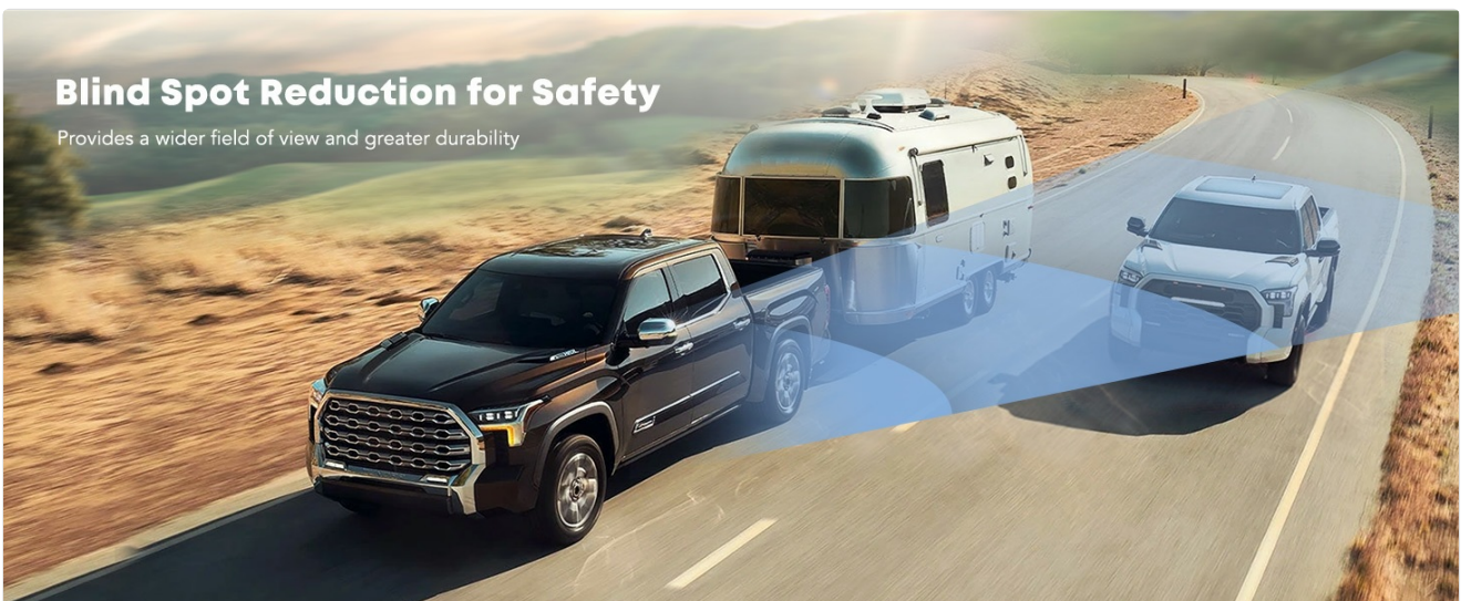
Image 8: Visualizing blind spot reduction, showing how the extended mirrors provide a wider field of view, especially when towing.
