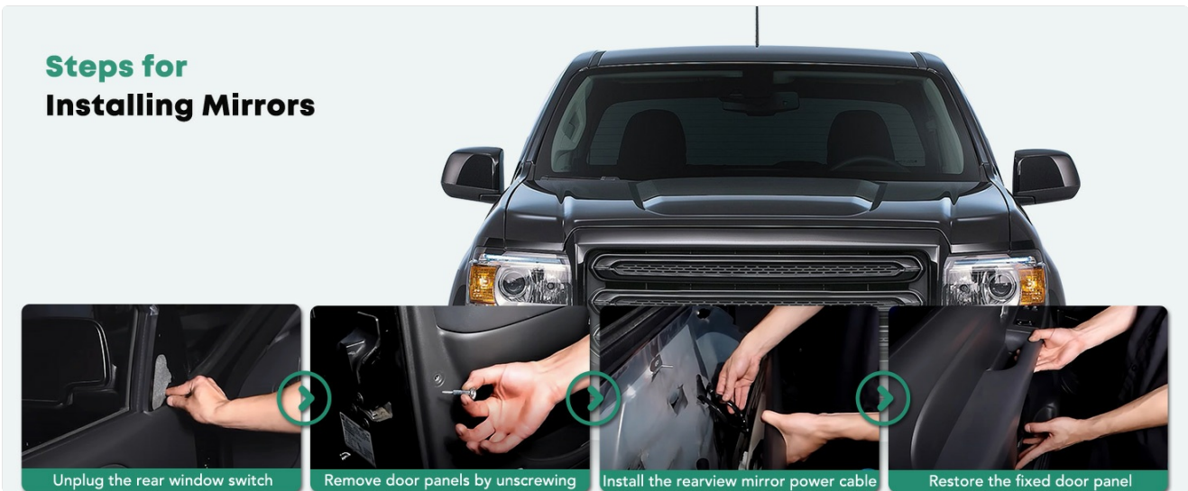
Image 5: Visual guide illustrating the general steps for mirror installation, including accessing the wiring and securing the new mirror.
