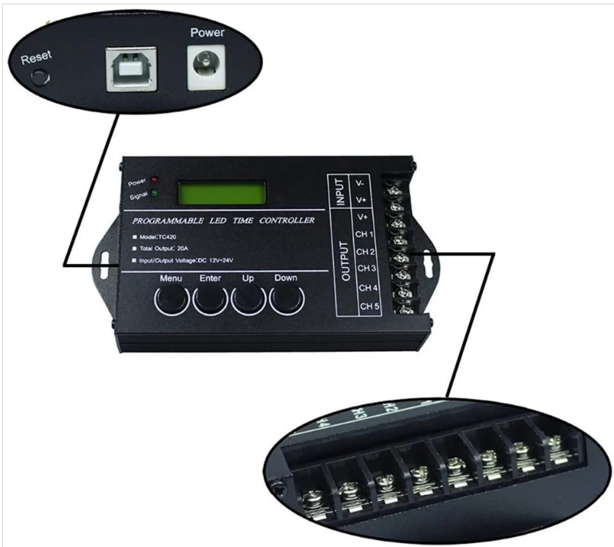
Figure 3: Detailed view of the CONTIA LED controller's connection ports. The top left shows the USB port for PC connection and the power input port. The bottom right shows the screw terminals for the 5 output channels (CH1-CH5) and the common anode (V+).
