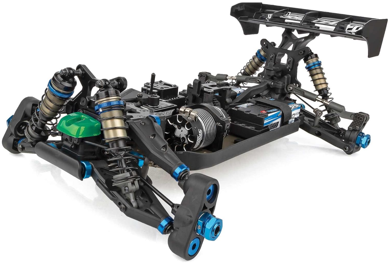
Figure 4.1: Detailed view of the RC8B4.1e's suspension and chassis components. This image highlights the shock absorbers, suspension arms, and drive shafts, which require regular inspection and maintenance.
