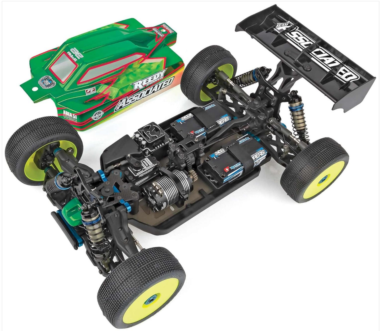
Figure 2.1: Chassis layout of the RC8B4.1e with the body removed. This view highlights the internal components, including the motor, batteries, and central differential, demonstrating the kit's modular design for assembly and customization.
