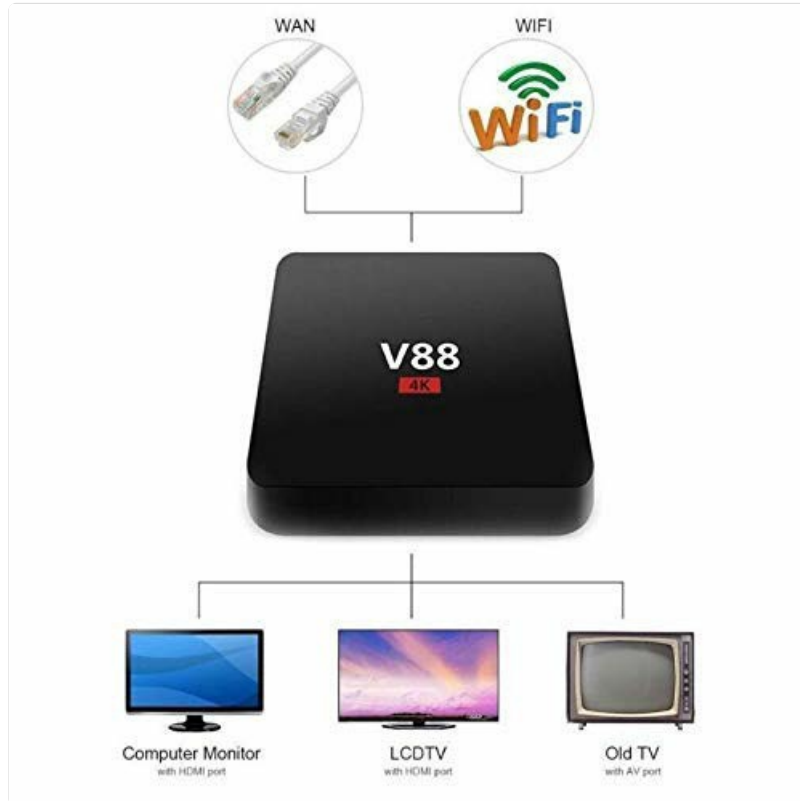
Figure 4.1: This diagram illustrates the various connectivity options for the V88R box, including WAN (Ethernet), WiFi, and output connections to a Computer Monitor (HDMI), LCDTV (HDMI), and Old TV (AV port).
