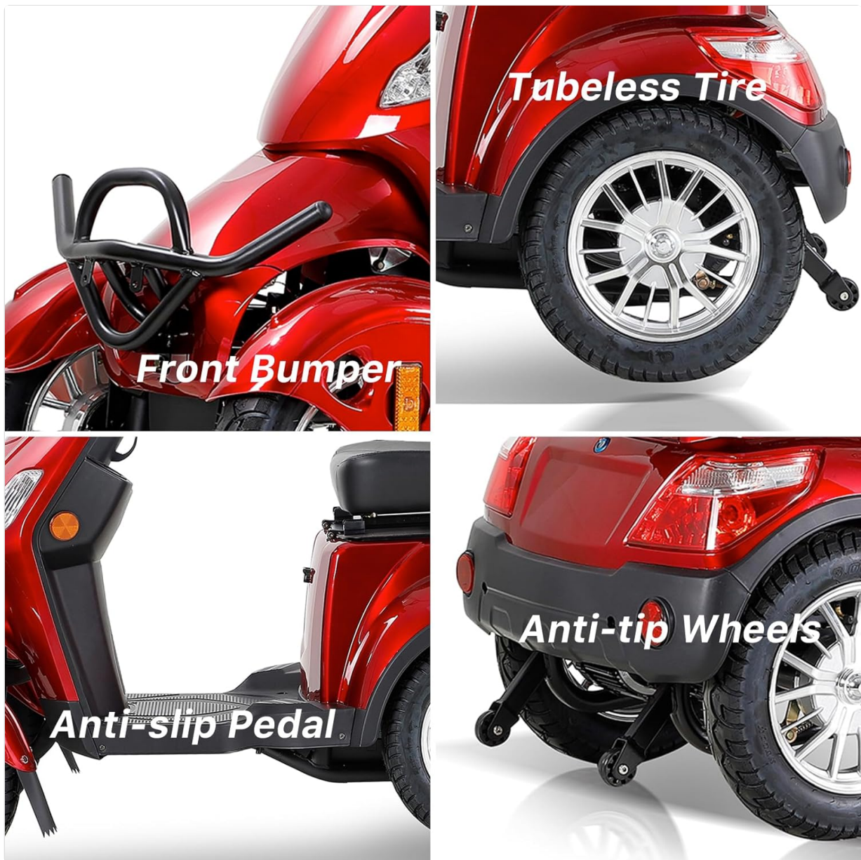
Image 2.1: Key safety and structural components of the scooter.
