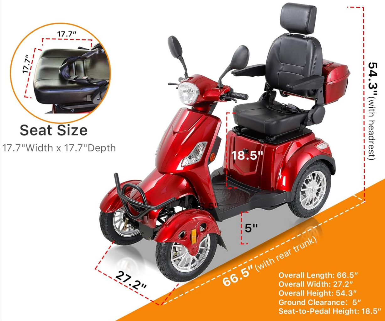
Image 10.1: Key dimensions of the scooter.
