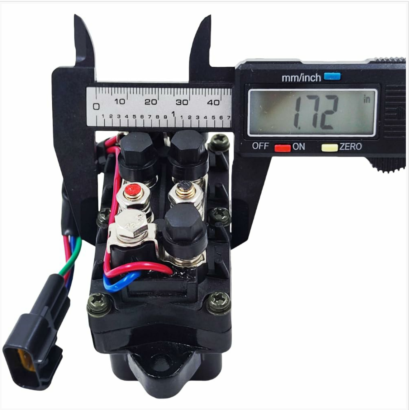
Figure 4.2: The solenoid relay with a digital caliper indicating a height of approximately 1.72 inches.
