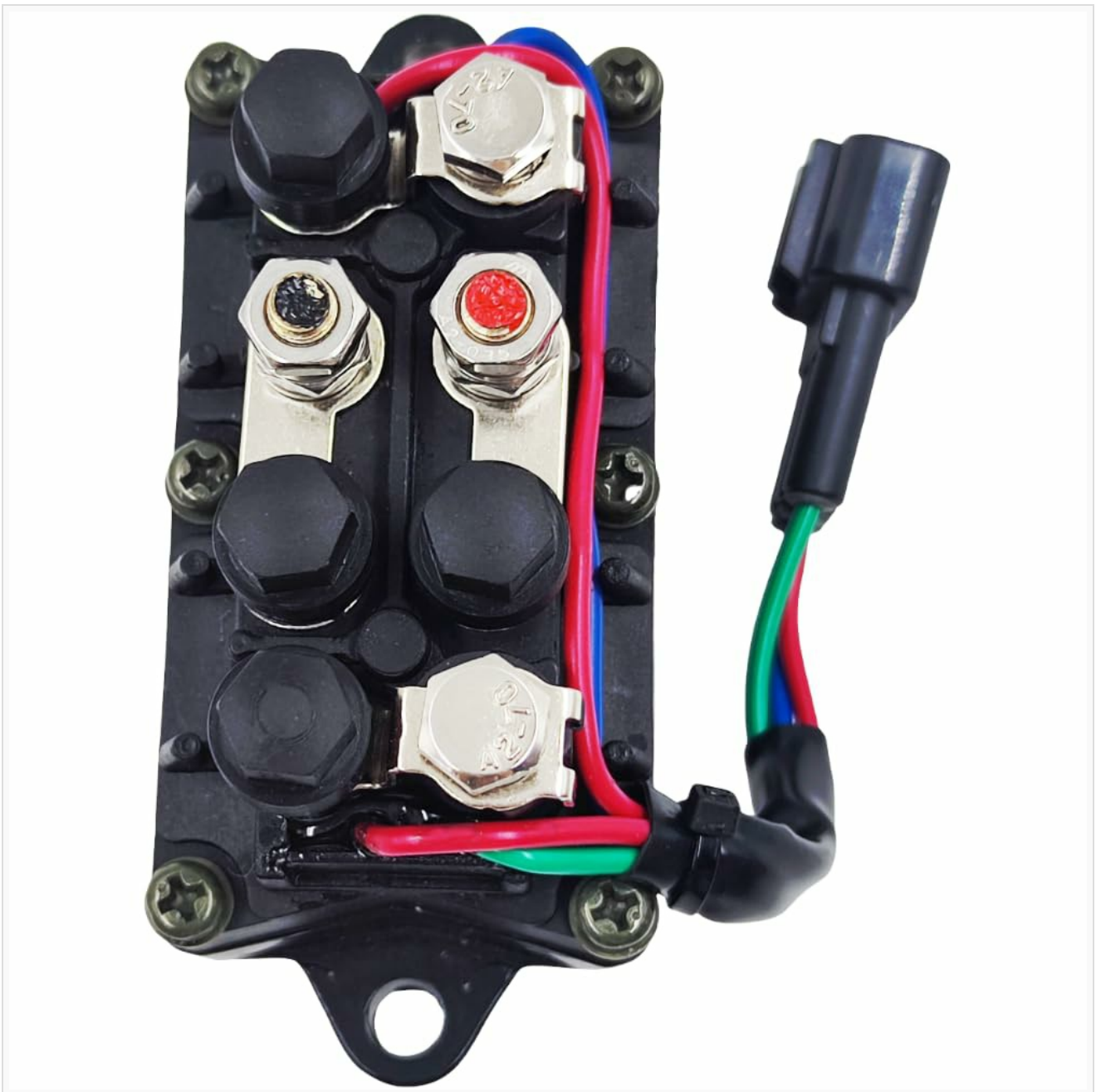
Figure 2.3: Top-down view of the solenoid relay, clearly showing the various terminals and their connections.
