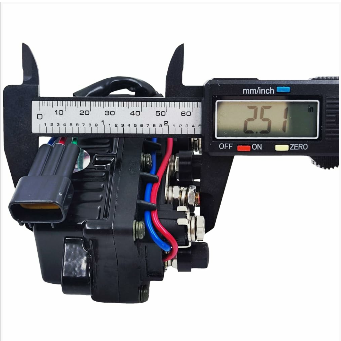
Figure 4.3: The solenoid relay with a digital caliper indicating a width of approximately 2.51 inches.
