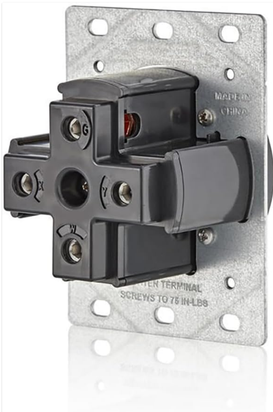
Image: Rear view of the Leviton 1450R receptacle, highlighting the G (Ground), W (Neutral), X (Hot), and Y (Hot)
