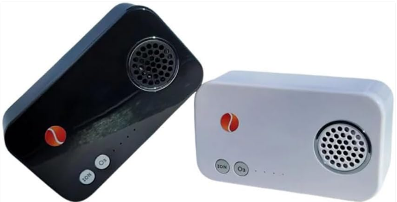
Figure 2: Close-up view of the black Therasage TheraO3 Ozone Module. This image highlights the 'ION' and 'O3' control buttons, the indicator lights, and the ozone/ion output grille.
