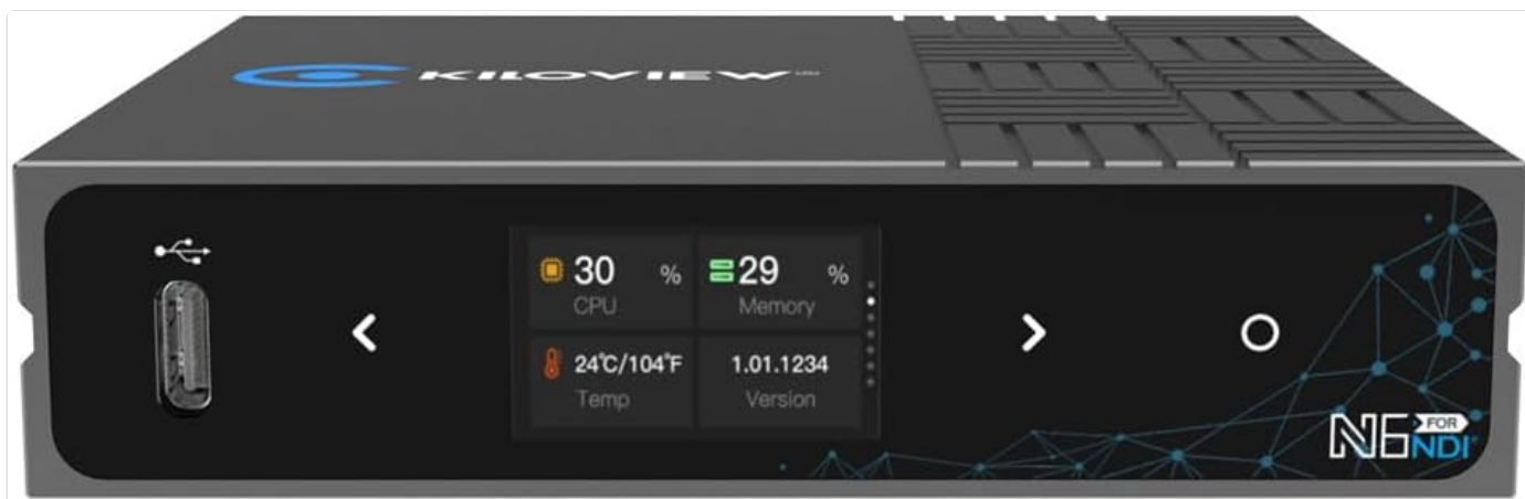
Figure 1: Front view of the Kiloview N6, showing the integrated 1.14-inch LCD screen which displays real-time status information such as CPU usage, memory, temperature, firmware version, and tally status. Navigation buttons are located on either side of the screen.
